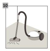
Directly before installation, the substrate should be carefully vacuumed to remove all dirt.
