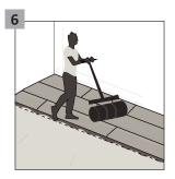
Immediately after laying three rows of panels, use a 50 kg roller to press them precisely and evenly to the ground. Rolling too late or improperly pressing hard-to-reach places may result in lack of proper adhesion and the panels sticking out from the substrate at the edges. It is recommended to re-roll the installed floor every 50 m<sup>2</sup>.
