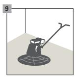
If a self-leveling compound is used, it is necessary to grind the surface to level it and remove the top layer.
