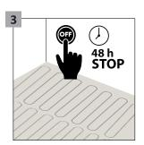
48 hours before installation, turn off the underfloor heating and, if necessary to maintain the guidelines regarding subfloor temperature and humidity, set the floor temperature to 18-20°C or use an alternative heating source.
