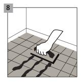
In case of installation on a surface covered with ceramic tiles, it is necessary to fill the joints of the tiles with a durable joint filling compound. Additionally, it is required to use a self-leveling compound to obtain a smooth surface with uniform absorbency.
