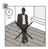
If the panels are installed to the substrate using an adhesive, heavy objects may be placed only after 72 hours from the gluing process, and the floor may be walked on gently after 4 hours from the gluing process.
